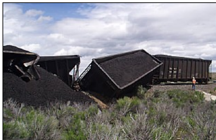
On May 18th, 2005, a derailment of 15 coal cars occurred near the propane off-loading site at the eastern edge of the City of Carlin. A sheared hub caused the wreck of the freight train on the west bound Union Pacific track. Photo: Laurel Marshall, Eureka County
