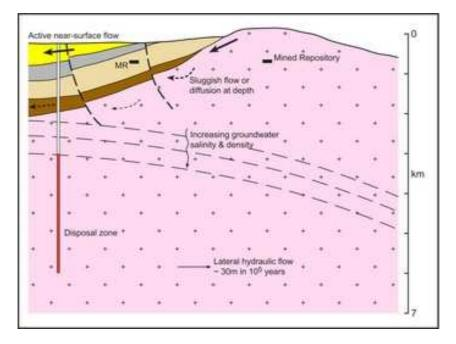
Figure 13. Deep Borehole Disposal Concept<sup>46</sup>
