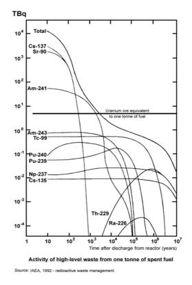
Figure 8. Radioactive Decay of Typical Spent Fuel
